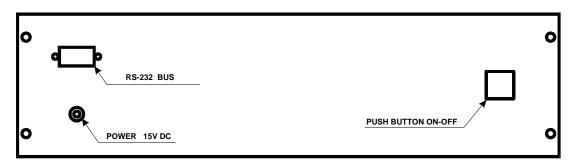
On the rear panel is the ON/OFF button for switching the decade on and off, supplying connector and a connector for connecting RS-232.
