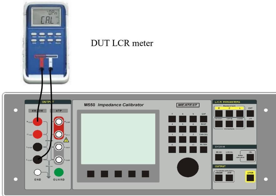
Figure 9 Two wire connection
