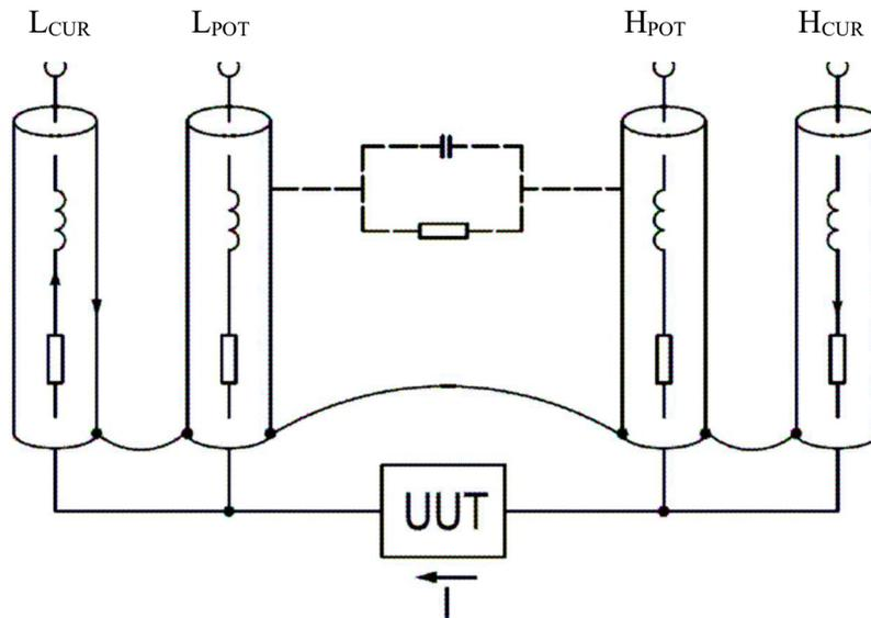
Figure 6 Principle of 4TP test lead connection
