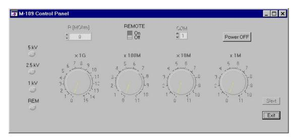
The light of indicating elements on the left-hand part of the screen is corresponding to LED diodes on the instrument panel. Rotary buttons on the control panel are displayed like "enable". They are only indicators of the real switches setup position on the front panel of the instrument now.
