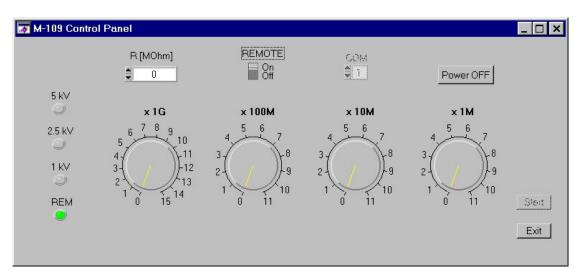
When supplying from a battery, you can switch off the instrument from the control panel by pressing the OFF button. This will break communication between the computer and the instrument.
