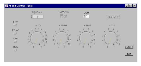
First use the operating element COM to select a serial port number to which the instrument is connected. Check if slide button REMOTE is in position OFF and confirm this selection using the START button. If the instrument is found on the serial line, actual instrument setup is read periodically and the setup of rotary buttons on the screen correspond to the setup on the instrument.
