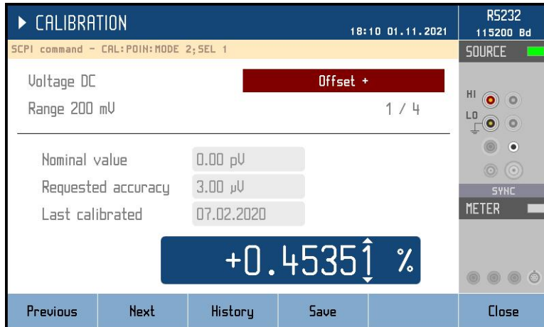
Figure 49 Calibration point adjustment - direct
